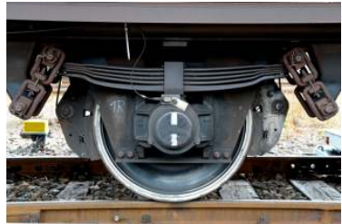
New LL brake blocks aimed to reduce noise from rail sector photo: UIC/EuropeTrain
