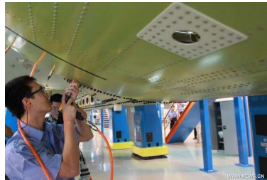
Fuselage of modern aircraft contains \approx 100\,000 rivets
