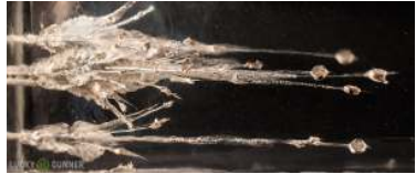
Handgun Self-Defense Ammunition Ballistics Test (bullet penetration in synthetic silicon)
