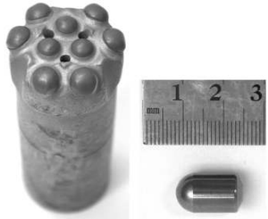
Drill crown and a single drill-bit button WC-Co
