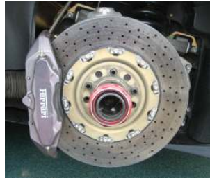
Reinforced carbon brake disc on a Ferrari F430 Wikipedia
