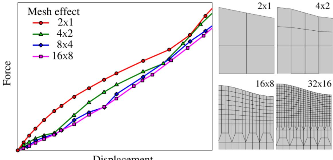
Fig. Effect of the mesh on mechanical response
