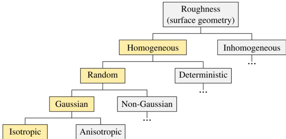
Fig. Roughness classification according to Nayak<sup>[1]</sup>
