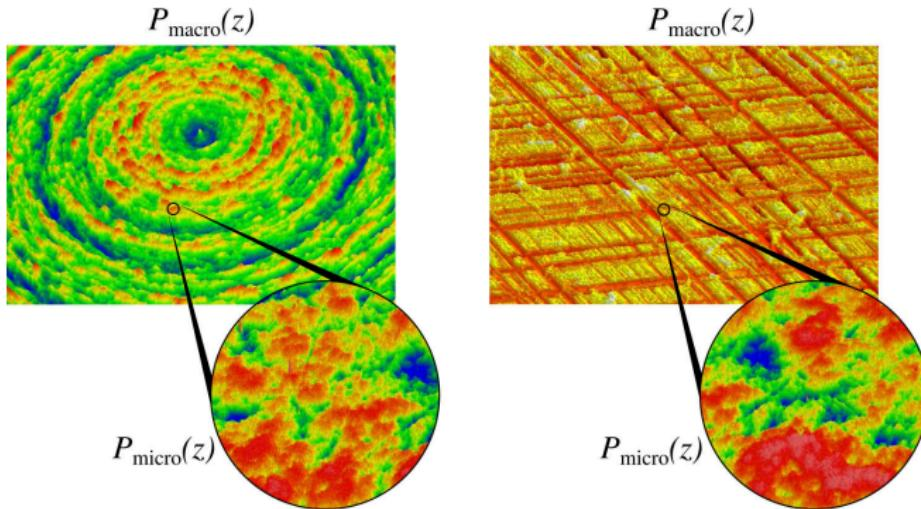
Macro- and microscopic roughness (left: diamond-turned surface, right: cross-hatched surface)
