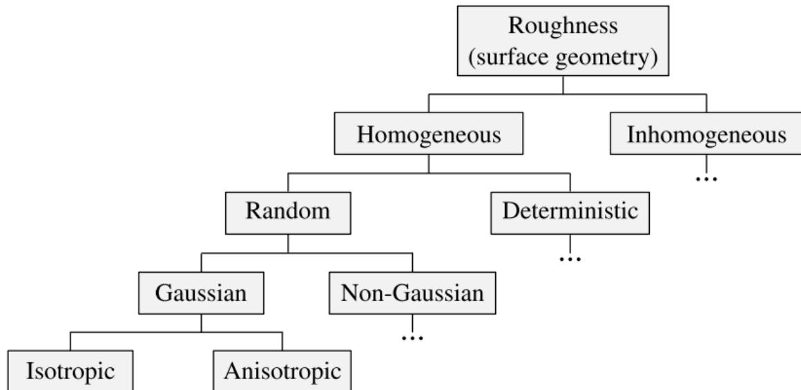
Fig. Roughness classification according to Nayak<sup>[1]</sup>
