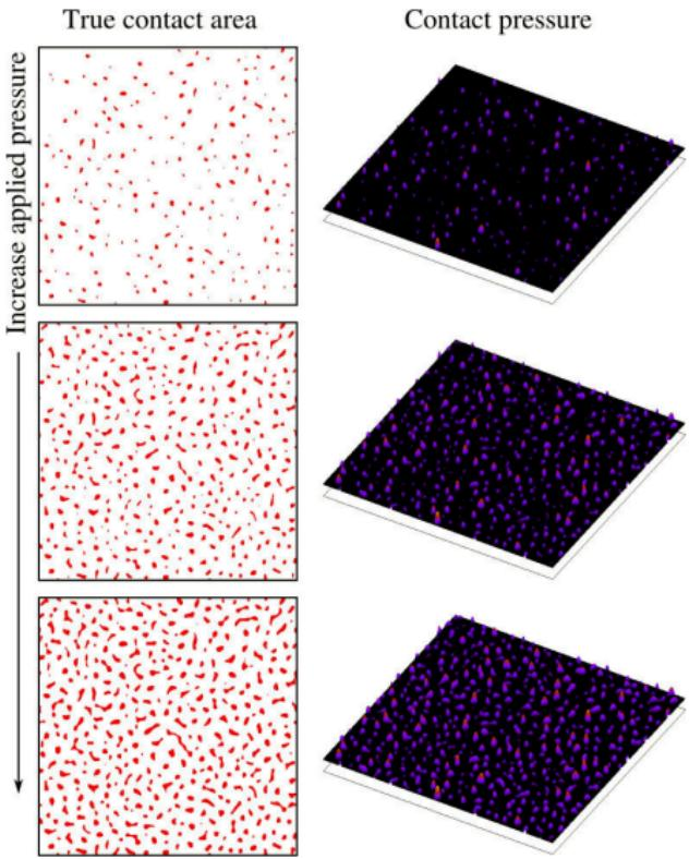
Fig. True contact area and stress fluctuations
