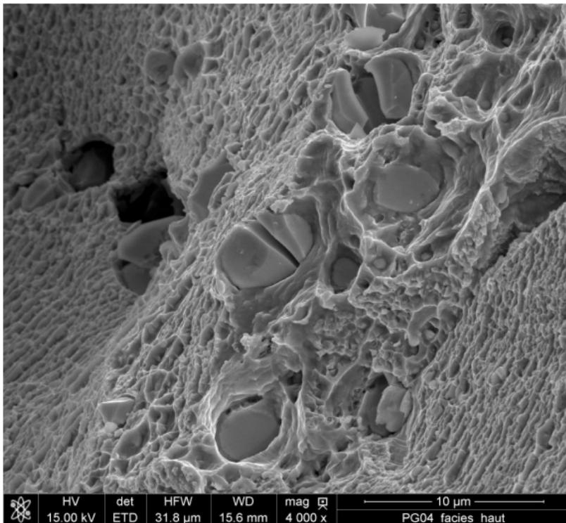
Fatigue fracture surface (Co-alloy), particles WC
