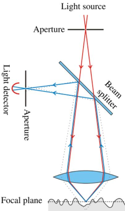
Principle of confocal microscopy
