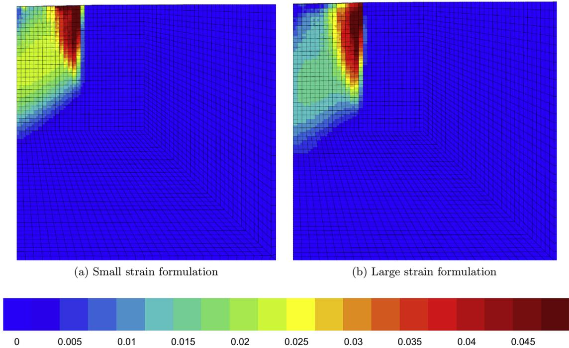
**Fig. 9.** Equivalent plastic strain field for FE computations using the small strain formulation of the model (b) and the finite deformation model (a), for Orientation A at a contact length of 140  $\mu\text{m}$ .
