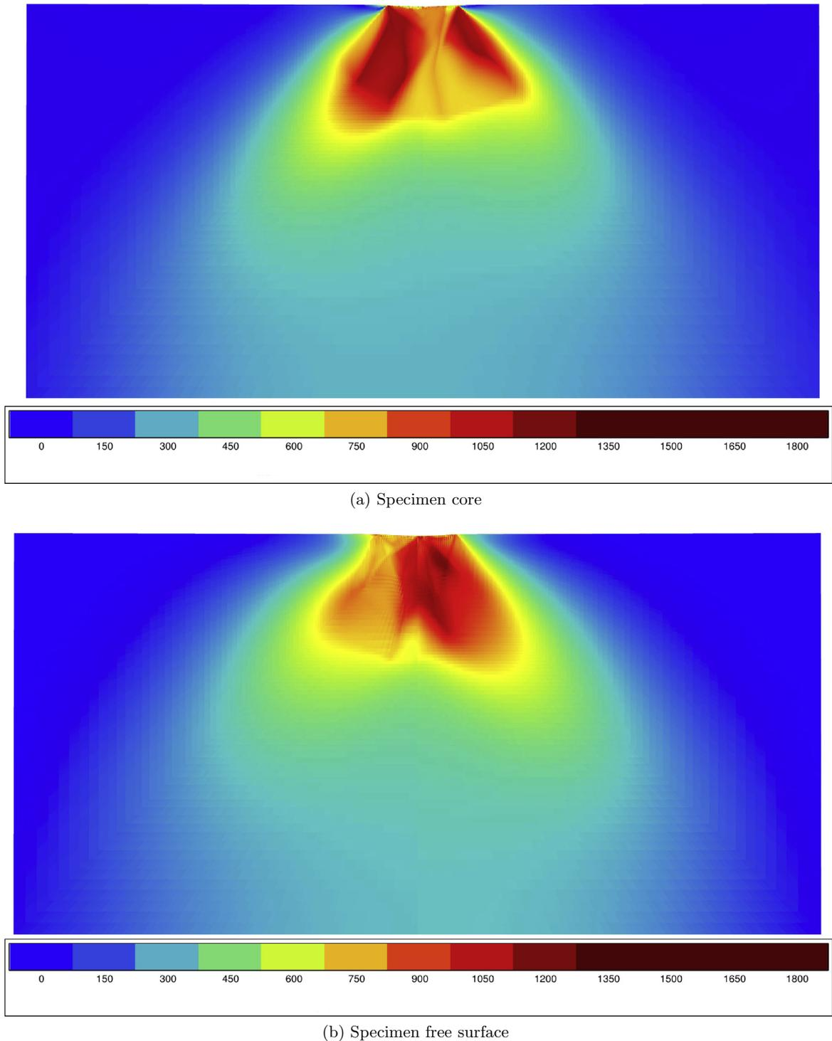
**Fig. 13.** Von Mises stress in Orientation A specimen.  $10^\circ$  misorientation was introduced for the simulation.
