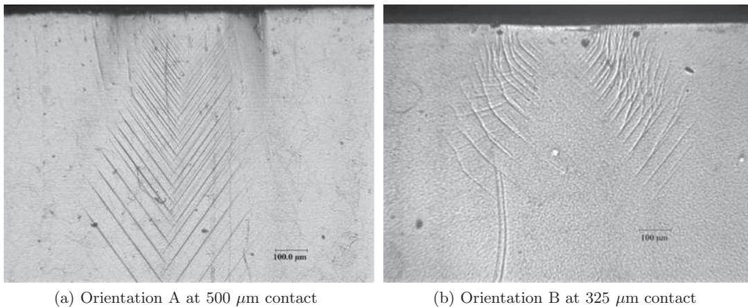
**Fig. 2.** Experimental slip traces observed.
