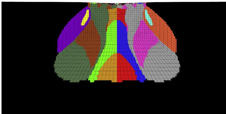
(b) Orientation B at 325  $\mu\text{m}$  contact length
