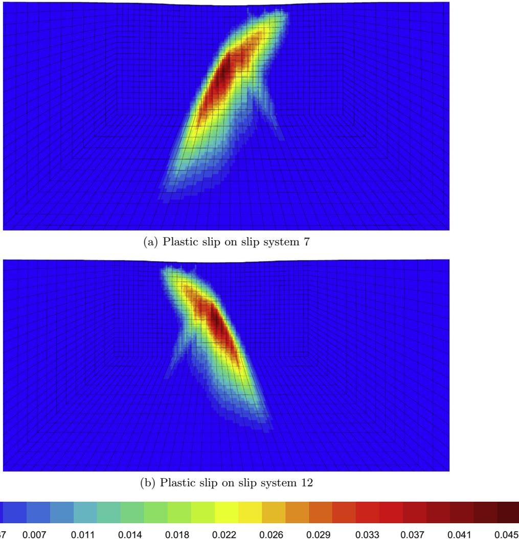
Fig. 7. Iso-values of plastic slip for systems 7 and 12 (orientation B).
