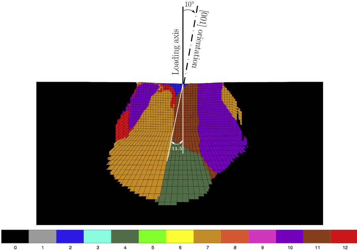
Fig. 12. Dominant slip map in specimen with Orientation A. A misorientation of 10° was introduced in the simulation.
