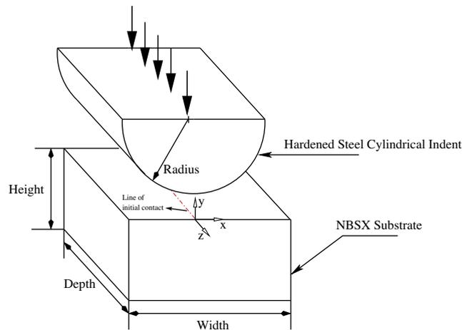
Fig. 1. Schematic representation of the indentation set-up.
