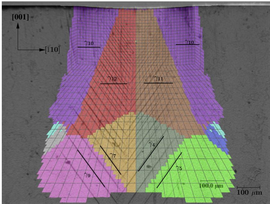
(a) Orientation A at 500 μm contact with indent
